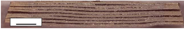
Fig. 3. Side view of a 16-layered, sintered tape cast S-morph structure, showing clear gaps between the layers due to the fugitive material. Scale bar = 1 mm.
